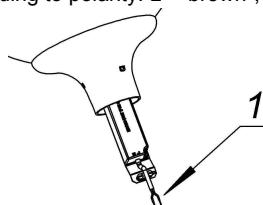
2. Lock mains cable (1) with strain relief (2) by screwing the screws (3).
