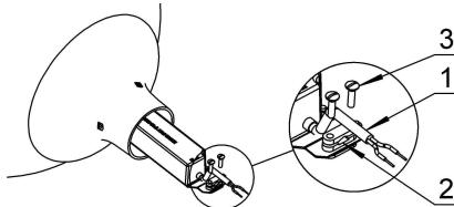
3. Place the luminaire on vertical support 60 mm in diameter, lock three screws (4). Tightening torque shouldn't exceed 4,5 Nm
