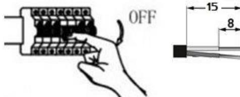
4. Connect mains cable to control gear's terminals according to scheme and polarity: "L" - phase conductor, "N" - negative conductor, the protective cover should be previously removed. Replace and secure control gear's protective cover.
