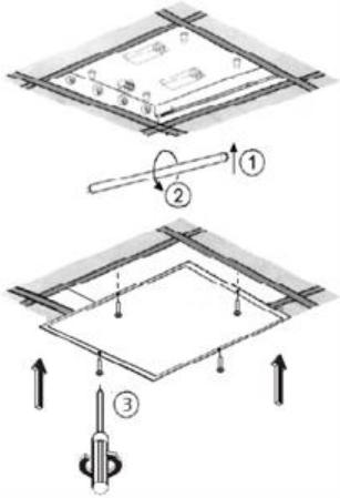
5. Put a lamp in. Fasten the glass on the luminaire housing
