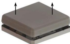
2. Put mains cable through bushing into luminaire's body, attach the body to bearing surface with X2 hardware kit (does not included), previously having put on screws metal washers and rubber rings (included).
