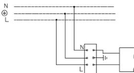
2. Mains connection scheme of luminaire with regulated control gear and ME6-NF unit.
