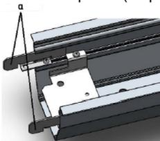
4. Suspend the luminaire on wires by putting wires through grippers (self-locking holders). Adjust height and horizontality of suspended luminaire
