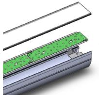
11. Replace assembly board back and lock it with screws.
